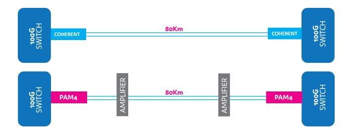
200Gbits and 400Gbits is a straightforward path thanks to Coherent and PAM4 technologies. The 100G is already a combination of 4x25Gbits (IM-DD) with direct detection. To keep a 25/28G baud rate, extra modulations are required combined with other components such as DSP.
