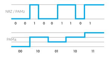
The main advantage of PAM4 is the easiness to use regular electronics and optical components suitable for small form factor such as QSFP28 from factor. The power consumption is drastically reduced and can be used for data centres interconnect application.
