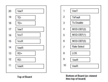
Pin-out of connector Block on Host board
