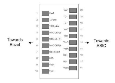
Pin-out of connector Block on Host board
