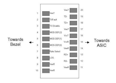
Pin-out of connector Block on Host board
