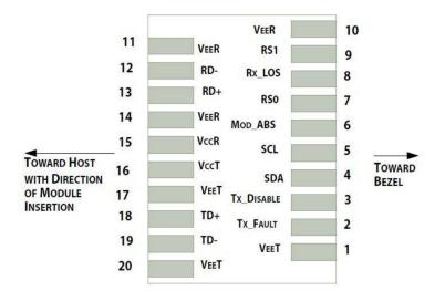
Pin-out of connector Block on Host board
