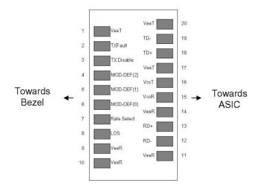
Pin-out of connector Block on Host board
