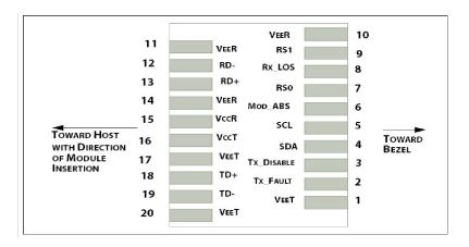
Pin-out of connector Block on Host board
