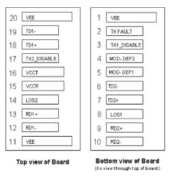
Pin-out of connector Block on Host board
