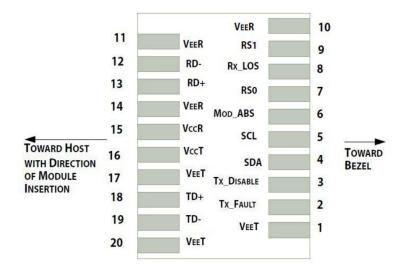
Pin-out of connector Block on Host board
