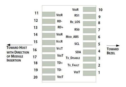
Pin-out of connector Block on Host board
