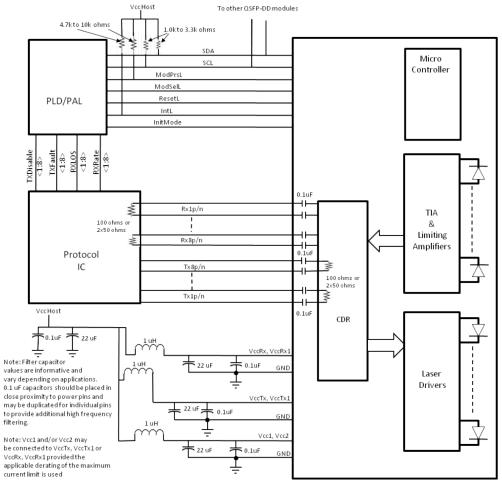
QSFP-DD Optical Module
