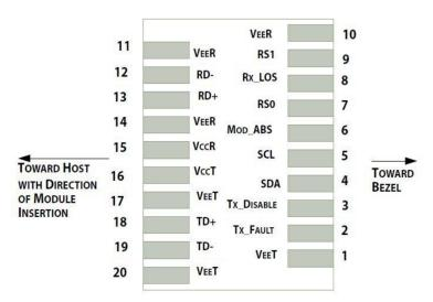
Pin-out of connector Block on Host board
