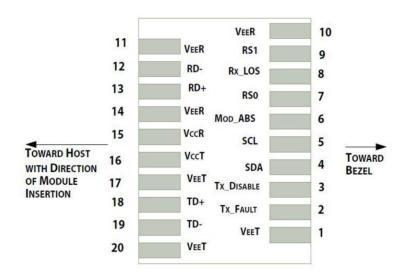
Pin-out of connector Block on Host board
