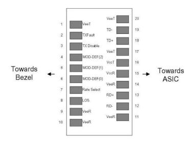
Pin-out of connector Block on Host board
