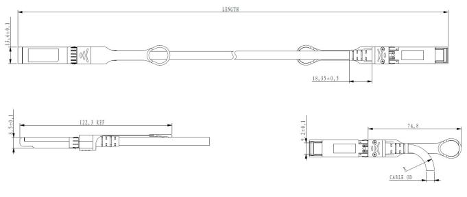
Unmarked Tolerance <u>+</u>0.2 Unit: mm
