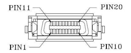
Pin-out of connector Block on Host board
