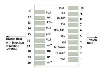
Pin-out of connector Block on Host board
