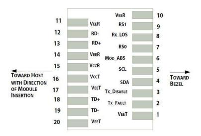
Pin-out of connector Block on Host board
