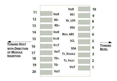
Pin-out of connector Block on Host board
