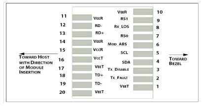
Pin-out of connector Block on Host board
