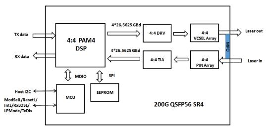
*Transmitter Section:* This module converts 4-channel 53.125Gbps electrical data to 4-channel 850nm 53.125Gbps optical signals for 212Gbps optical transmission.
