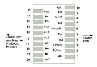
Pin-out of connector Block on Host board
