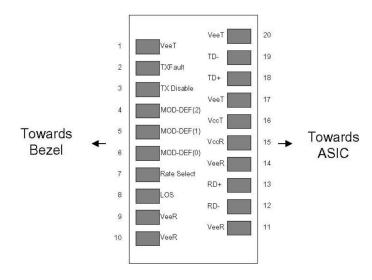
Pin-out of connector Block on Host board
