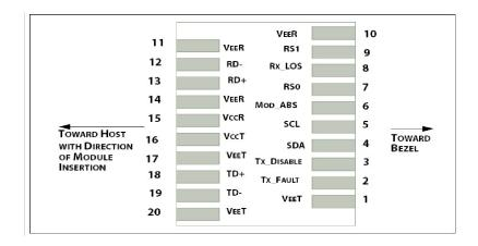
Pin-out of connector Block on Host board
