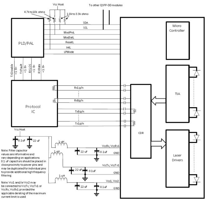
QSFP-DD Optical Module
