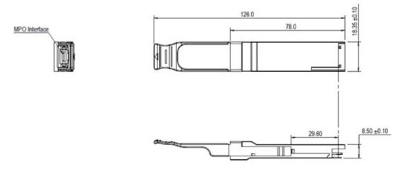
**Attention:** To minimize MPO connection induced reflections, an MPO receptacle with 8-degree angled end-face is utilized for this product. A female MPO connector with 8-degree end-face should be used with this product as illustrated in below Figure.
