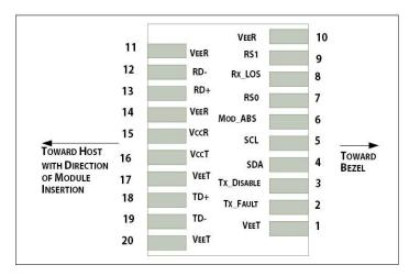
Host PCB SFP56 Pad Assignment Top View
