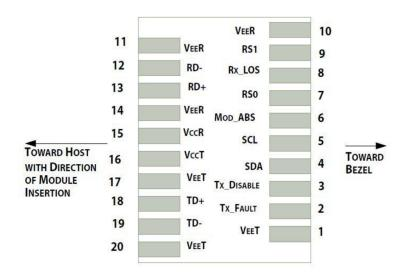
Pin-out of connector Block on Host board
