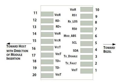
Pin-out of connector Block on Host board
