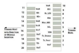
Pin-out of connector Block on Host board
