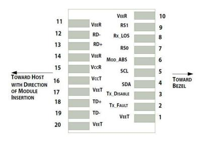
Pin-out of connector Block on Host board
