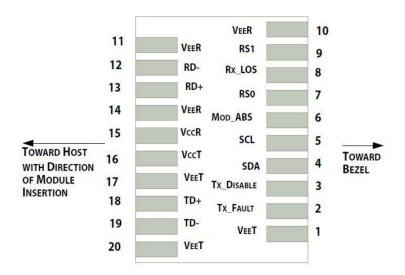
Pin-out of connector Block on Host board
