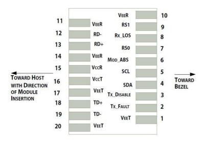
Pin-out of connector Block on Host board
