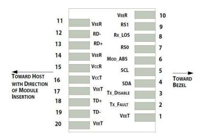
Pin-out of connector Block on Host board
