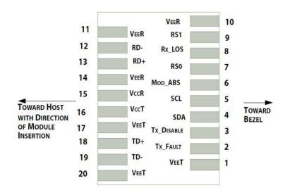
Pin-out of connector Block on Host board
