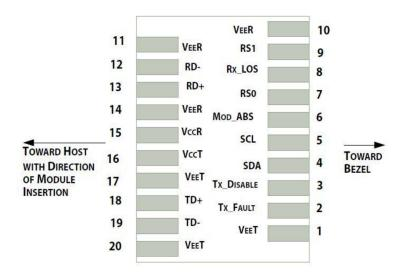
Pin-out of connector Block on Host board
