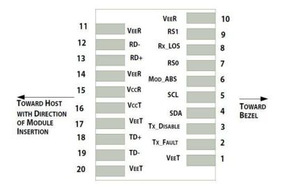
Pin-out of connector Block on Host board
