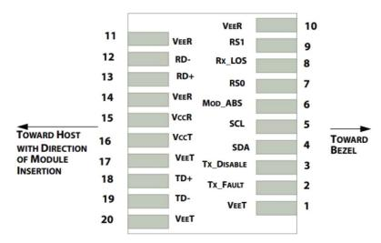
**Electrical Pin-out Details for SFP**
