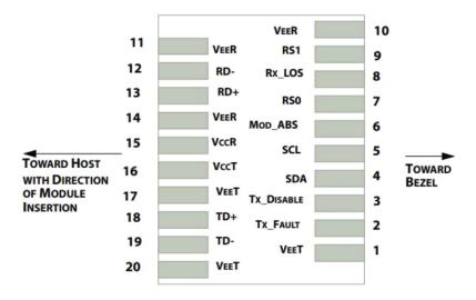
**Electrical Pin-out Details for SFP**
