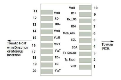
Pin-out of connector Block on Host board
