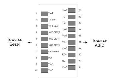
Pin-out of connector Block on Host board
