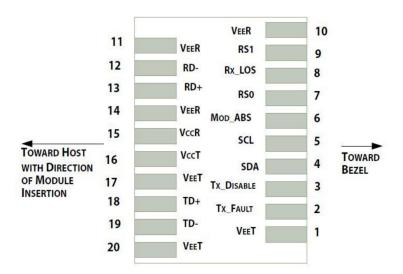
Pin-out of connector Block on Host board
