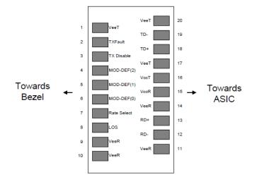
Pin-out of connector Block on Host board
