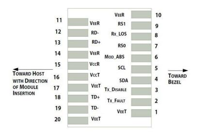
Pin-out of connector Block on Host board
