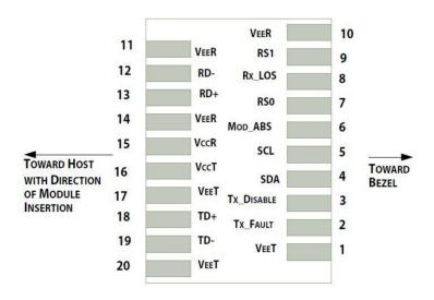
Pin-out of connector Block on Host board
