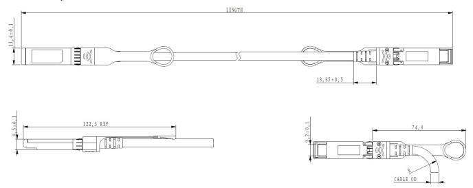
Unmarked Tolerance <u>+</u>0.2 Unit: mm
