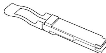
QSFP28 PAM4 80km DWDM 100Ghz "Super Channel" 4.5W (require amplifier).
