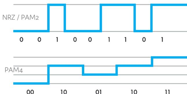
The main advantage of PAM4 is the easiness to use regular electronics and optical components suitable for small form factor such as QSFP28 form factor. The power consumption is drastically reduced and can be used for data centres interconnect application.
