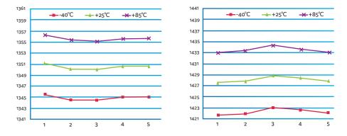
The WDM transceiver with the 1351nm center wavelength drifted between just short of 1357nm at high temperature down to 1345nm at low temperature in this study. Whereas, the 1431nm transceiver experiences a much wider drift, down to 1421nm at low temperature.
